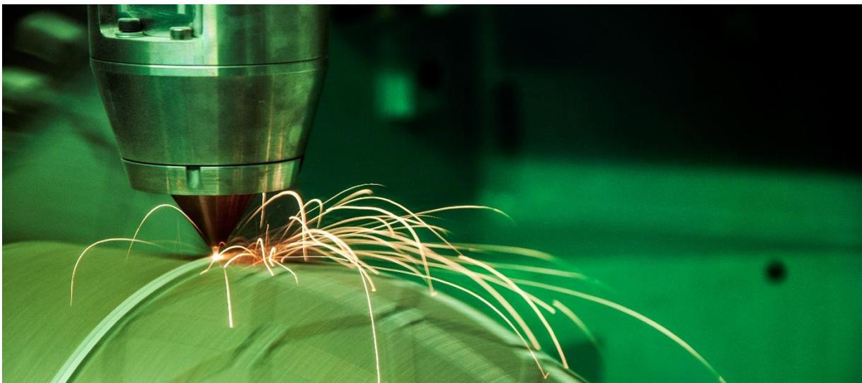
*DED is an Additive Manufacturing process where focused thermal energy is used to fuse materials by melting them as they are deposited.*
